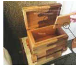
➔ Ben's '50/50' box, made from oak and walnut, features a secret compartment – see photo annotations above
